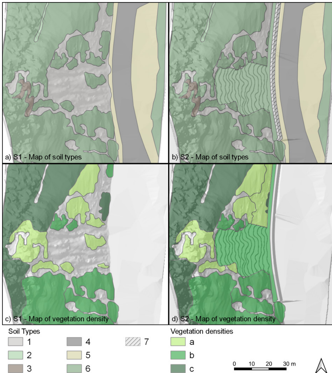
Figure 61: Input maps used for rockfall simulation with RAMMS::Rockfall varying for the two modelled scenarios S1 and S2, including hill-shaded background showing ante opera and post opera slope morphology: a) Mapped soil types for S1; b) Mapped soil types for S2, according to the project layout; c) Mapped vegetation densities for S1; c) Mapped vegetation densities for S2.
