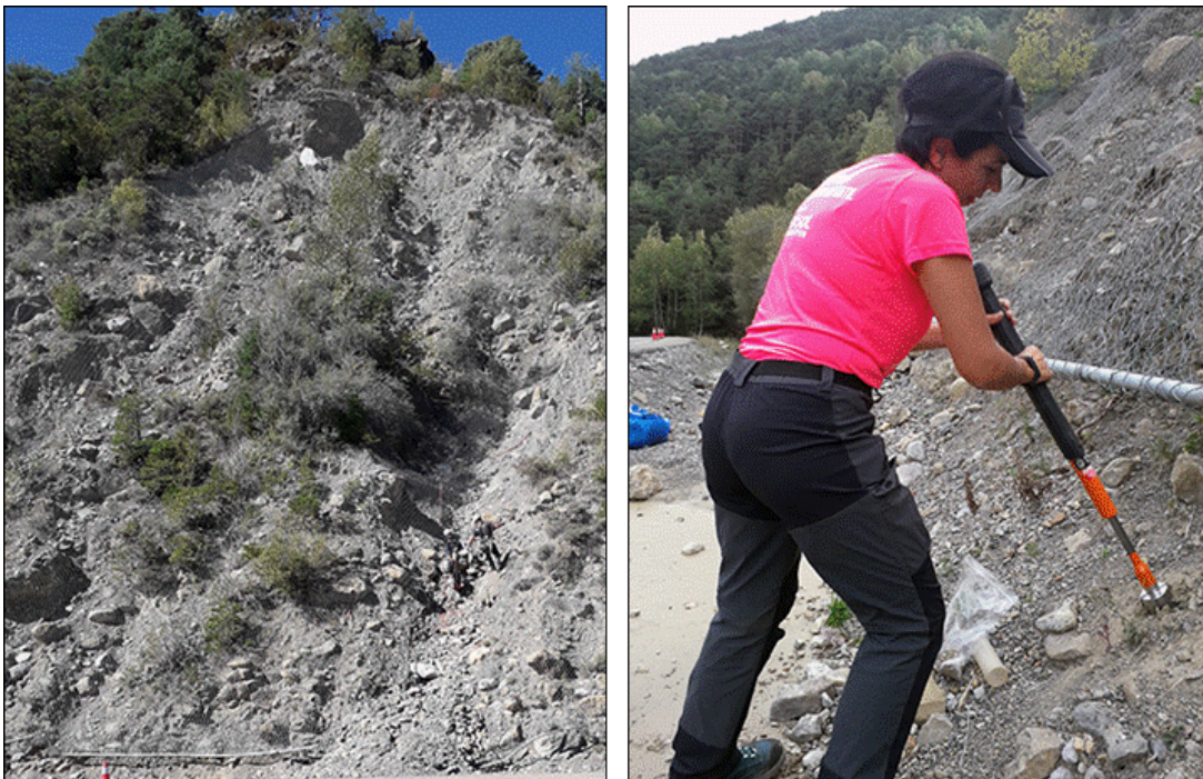
Figure 17. Soil sampling in the Santa Elena road cut
